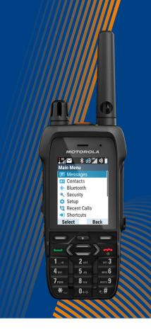
The MXP660 is a rugged and lightweight, yet fully capable, TETRA portable radio with built-in LTE that's easy to carry and easy to use. So that vital messages get through, the MXP660 has the option to ramp up to Class 3 TETRA transmission power. If an MXP660 user goes outside of TETRA coverage, the radio can automatically switch to available LTE or Wi-Fi broadband, maintaining DIMETRA™ features and workflows via DIMETRA Connect.
